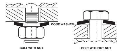
The Spring Cone Washers are installed under the **NUT** and the nut tightened to the torque installation recommendations above. If the bolt is not a through bolt, the washer should be installed under the **BOLT HEAD** and the bolt tightened to the proper values. Alternate tightening of bolts from side to side and top to bottom. The small end of the Spring Cone Washer should be against the nut or bolt head. (see illustrations)
