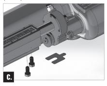
7. Replace the shims under the travel indicator in the same position as removed in step 4 (**Pic. D**).
