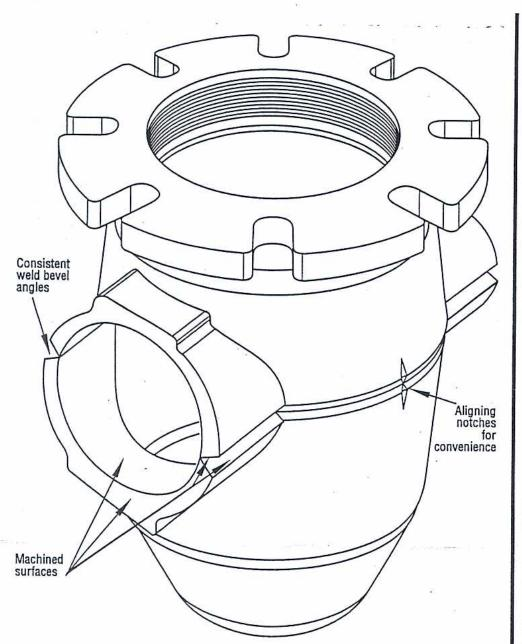
The enhanced design of Mueller's Line Stopper Fittings features machined surfaces on all contact points between the pipe and the fitting, lateral weld seams and interior stopper landing surfaces. Machined surfaces provide consistent weld land widths, consistent bevel angles and accurate positioning of stoppers for better first time sealing.
